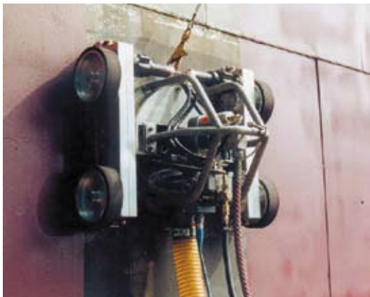
Lizard with remote control for emissions-free large-scale surface preparation
