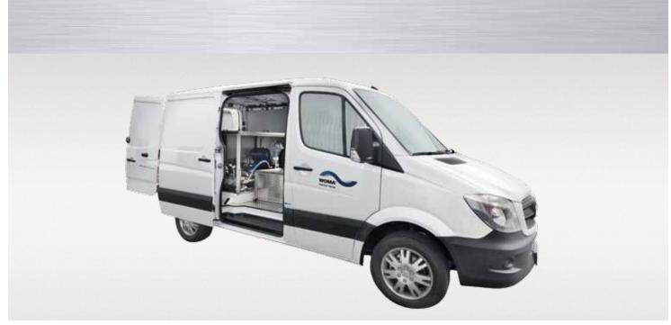
The new EcoRunner quickly delivers high pressure where it is needed. The vehicle and water jet combination unites transport and operation of ultra high pressure technology in one device. This modular design enables quick and flexible conversion for all high pressure water jetting applications.
