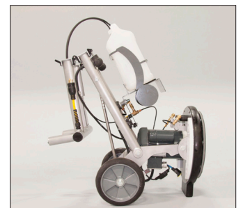
Folds down to 30" tall which makes it easy for transport and storage.
