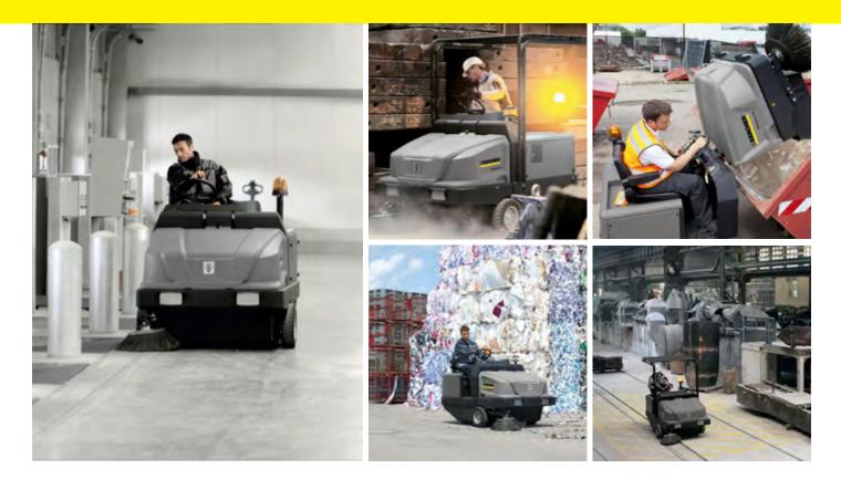
Kärcher sweepers offer large area performance, excellent cleaning results and numerous accessory options. They have different drive types for use in indoor areas, outdoor areas or both. Choose between one or two side brushes. Suction and advanced filter technologies for a dust-free environment. Larger ride-on sweepers have a hydraulic container lift for convenient high container emptying.
