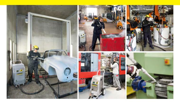
Do you want a way to remove stubborn dirt that is as effective as it is gentle? Then the Ice Blaster from Kärcher is the right solution for you. The system uses compressed air and dry ice pellets to remove rubber residues, oils, greases, parting agents, dyes etc. from workpieces or surfaces.
